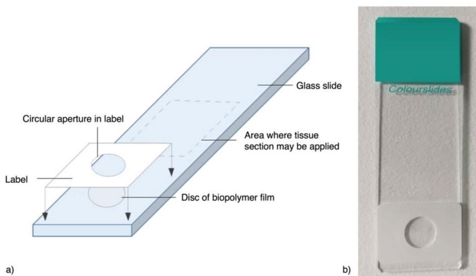
**Fig. 1** Stain assessment slide. An illustration (a) and a photo (b) of an example stain assessment slide, consisting of a disc of biopolymer film positioned onto a glass slide, with a chemically resistant PET label positioned on top to affix the biopolymer in position. The dotted grey line indicates the area where tissue sections may be mounted
