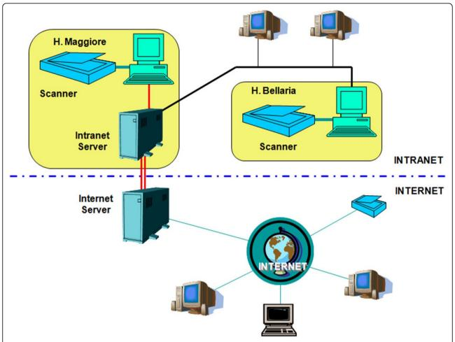
**Figure 1** Network scheme: two scanner are in an intranet environment with an local disk server, connected to an internet server where the public products are stored.
