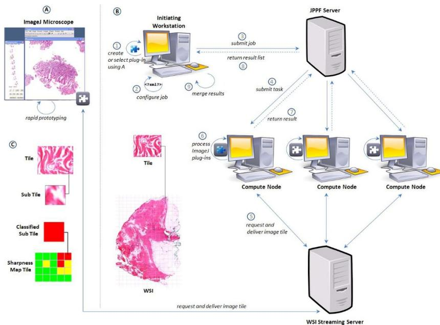
**Figure 2 System overview.** A) The ImageJ microscope can be used for rapid prototyping purposes. B) An image processing job is divided into several tasks. Image tiles are processed on a grid of standard PCs (compute nodes). Each node receives image tiles and processes predefined plug-ins. Results are merged using a domain specific implementation. C) Application to sharpness assessment.
