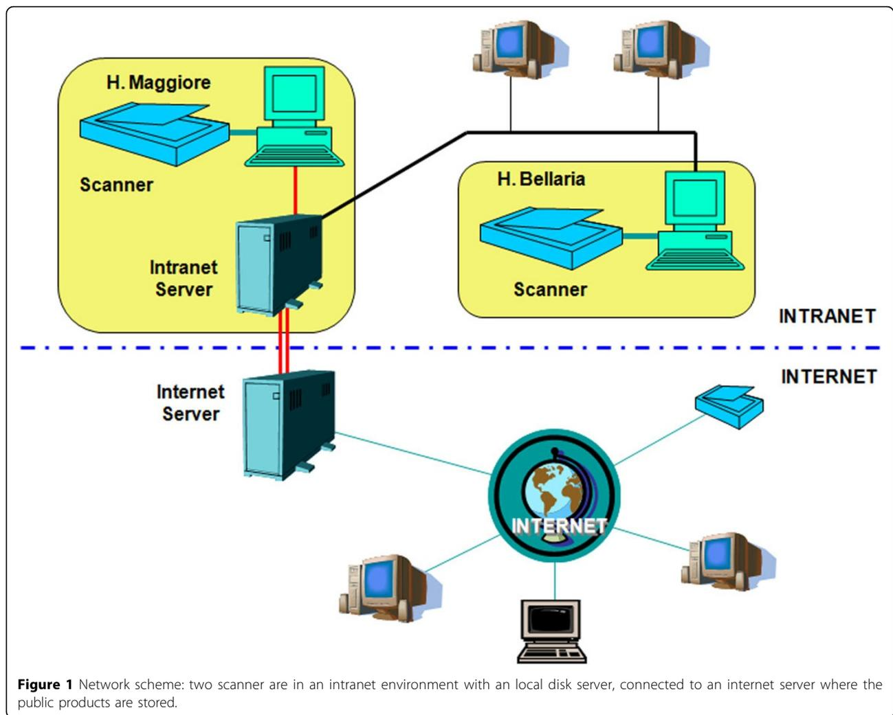
**Figure 1** Network scheme: two scanner are in an intranet environment with an local disk server, connected to an internet server where the public products are stored.
